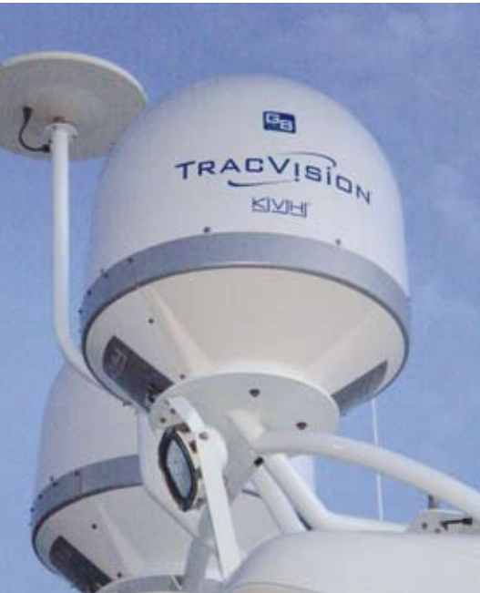
This picture: Satellite communications receiver used for picking up TV, Internet and phone any place on the ocean. Different system than a GPS but similar satellite principle.
